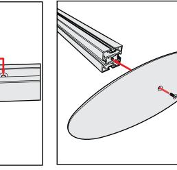
Base Plate & Extrusion Connection
